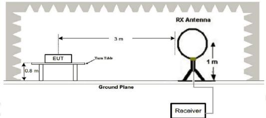
2. Radiated Emission Test-Up Frequency 30MHz~1GHz
