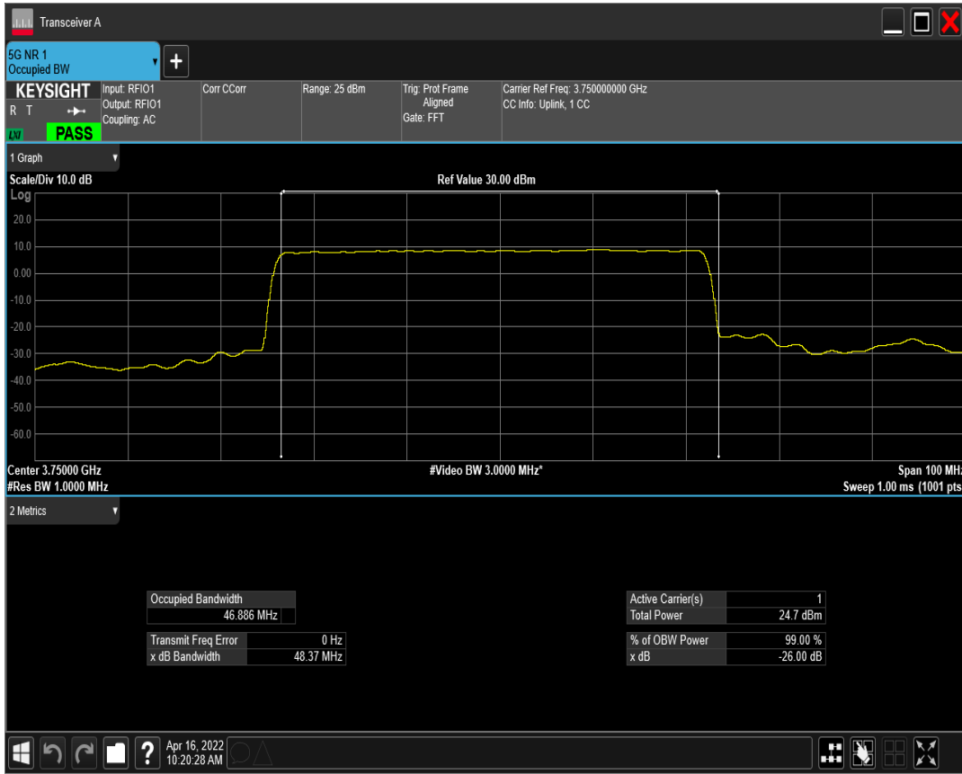
n78(3700-3800) SCS=30kHz DFT_QPSK BW=50MHz Channel=650000 RB=128@0
