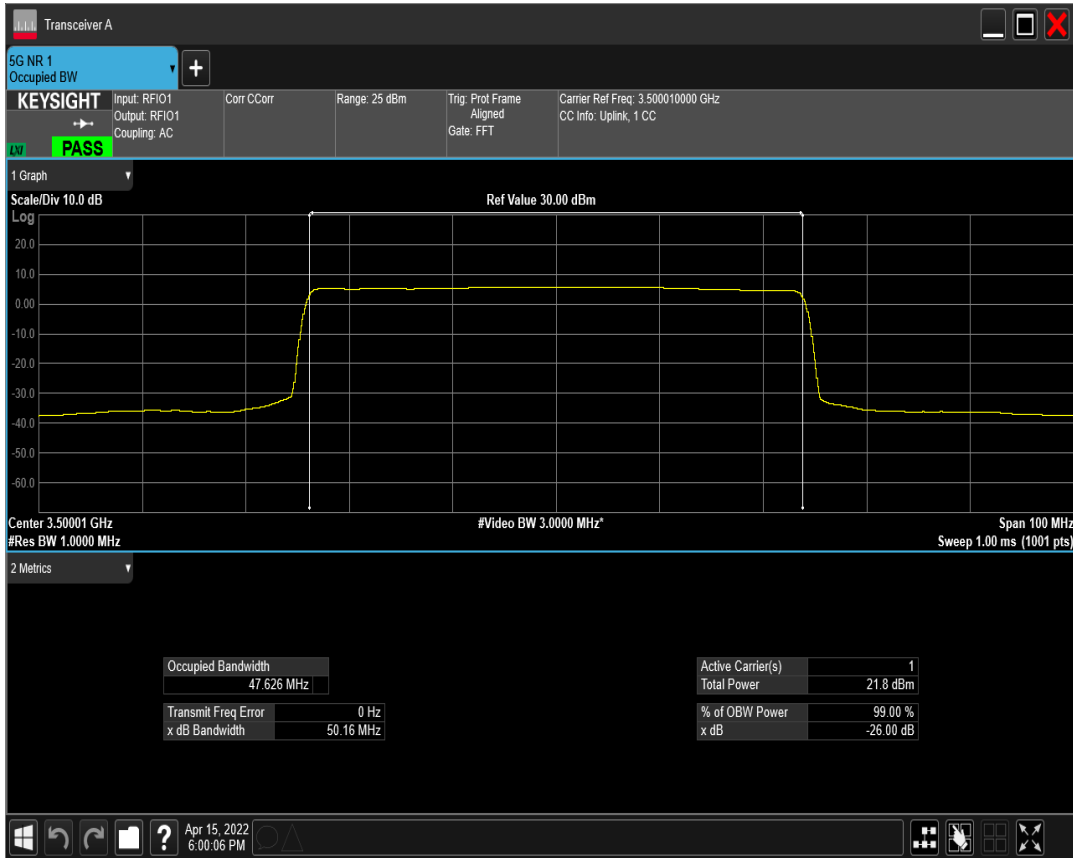
n78(3450-3550) SCS=30kHz DFT_BPSK BW=50MHz Channel=635000 RB=128@0
