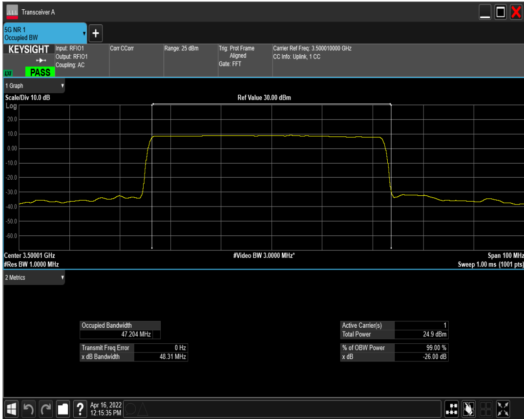
n78(3450-3550) SCS=30kHz DFT_QPSK BW=50MHz Channel=633334 RB=128@0
