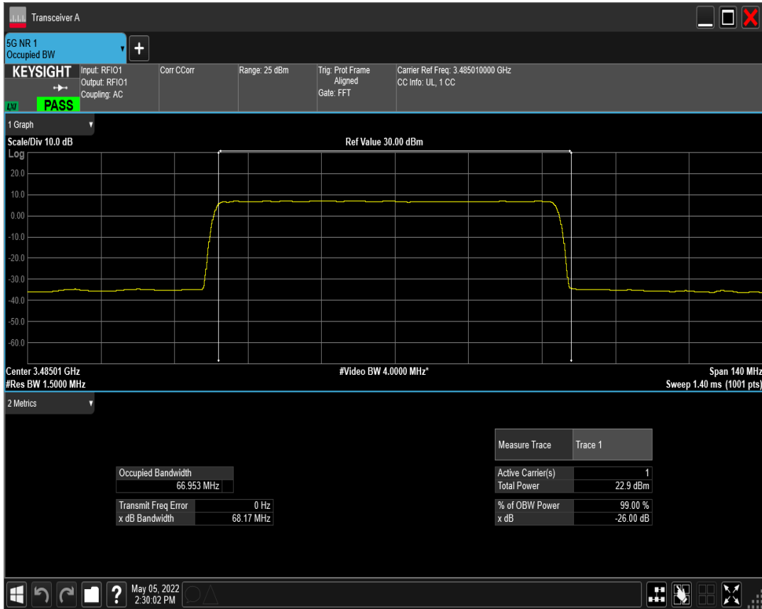
n78(3450-3550) SCS=30kHz DFT_QAM16 BW=70MHz Channel=634332 RB=180@0
