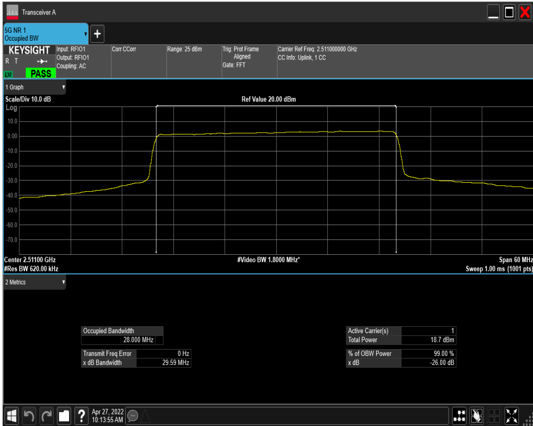
n41 SCS=30kHz CP_QAM64 BW=30MHz Channel=502200 RB=78@0 ant2
