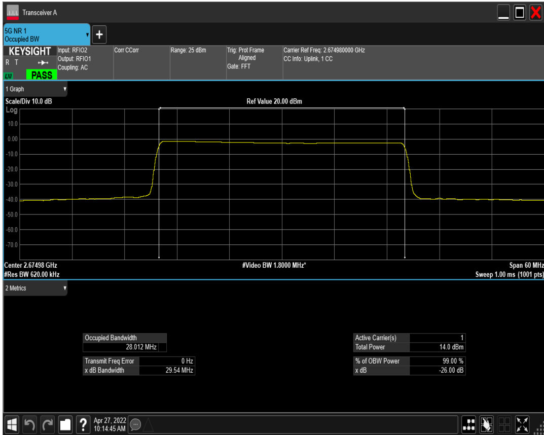
n41 SCS=30kHz CP_QAM16 BW=30MHz Channel=534996 RB=78@0 ant1
