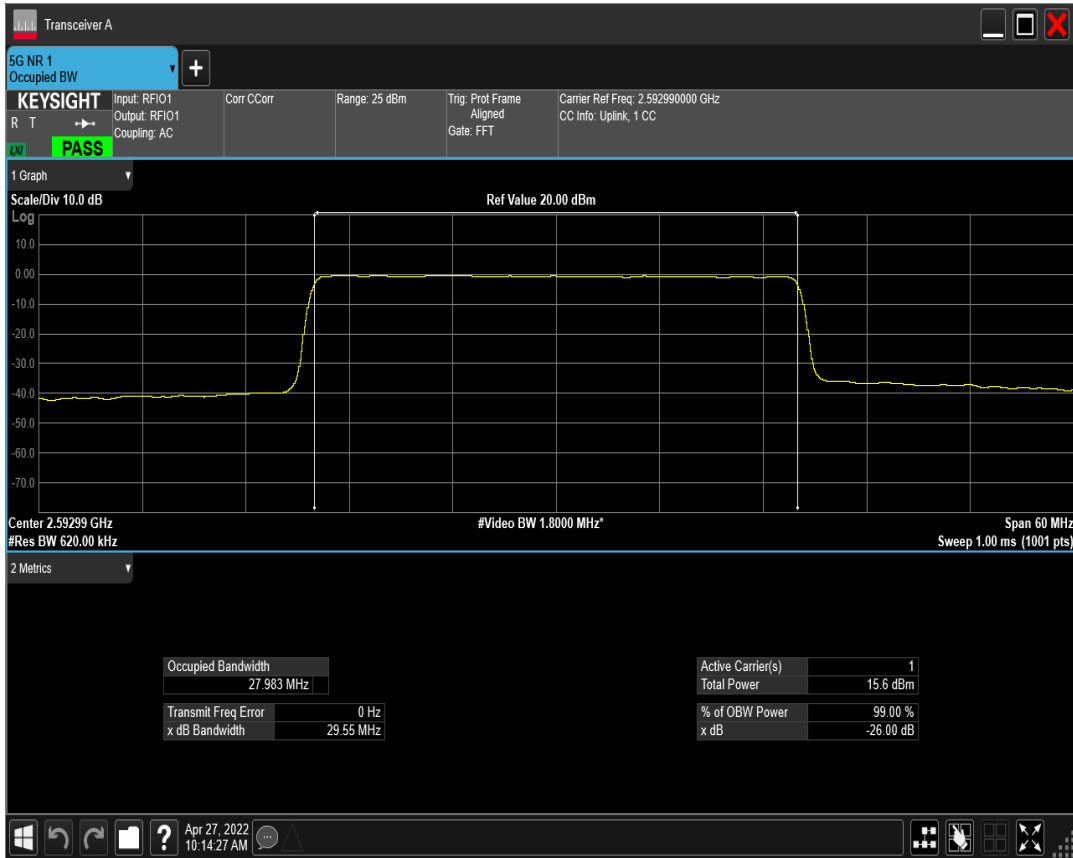
n41 SCS=30kHz CP_QAM256 BW=30MHz Channel=518598 RB=78@0 ant2
