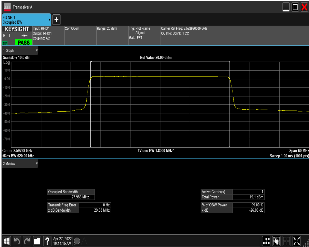
n41 SCS=30kHz CP_QPSK BW=30MHz Channel=518598 RB=78@0 ant2
