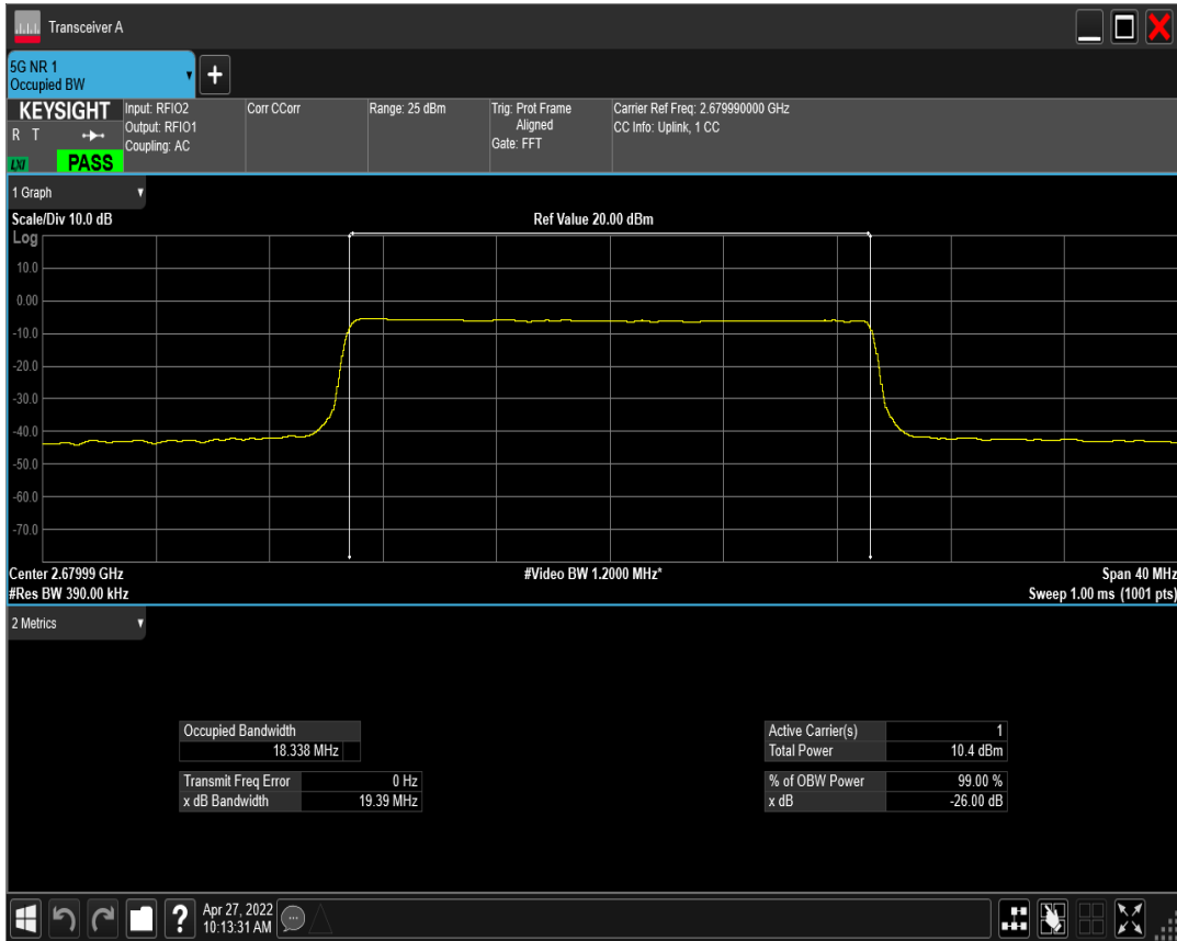
n41 SCS=30kHz CP_QPSK BW=30MHz Channel=502200 RB=78@0 ant1
