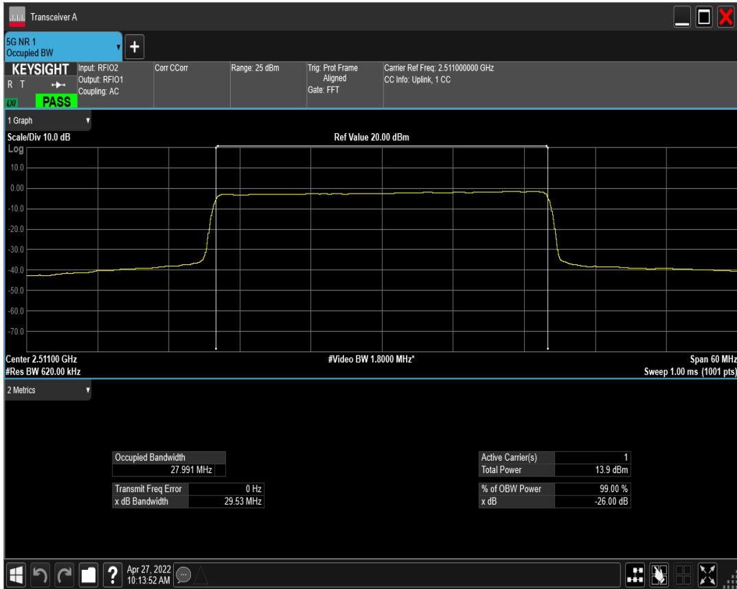
n41 SCS=30kHz CP_QAM64 BW=30MHz Channel=502200 RB=78@0 ant1
