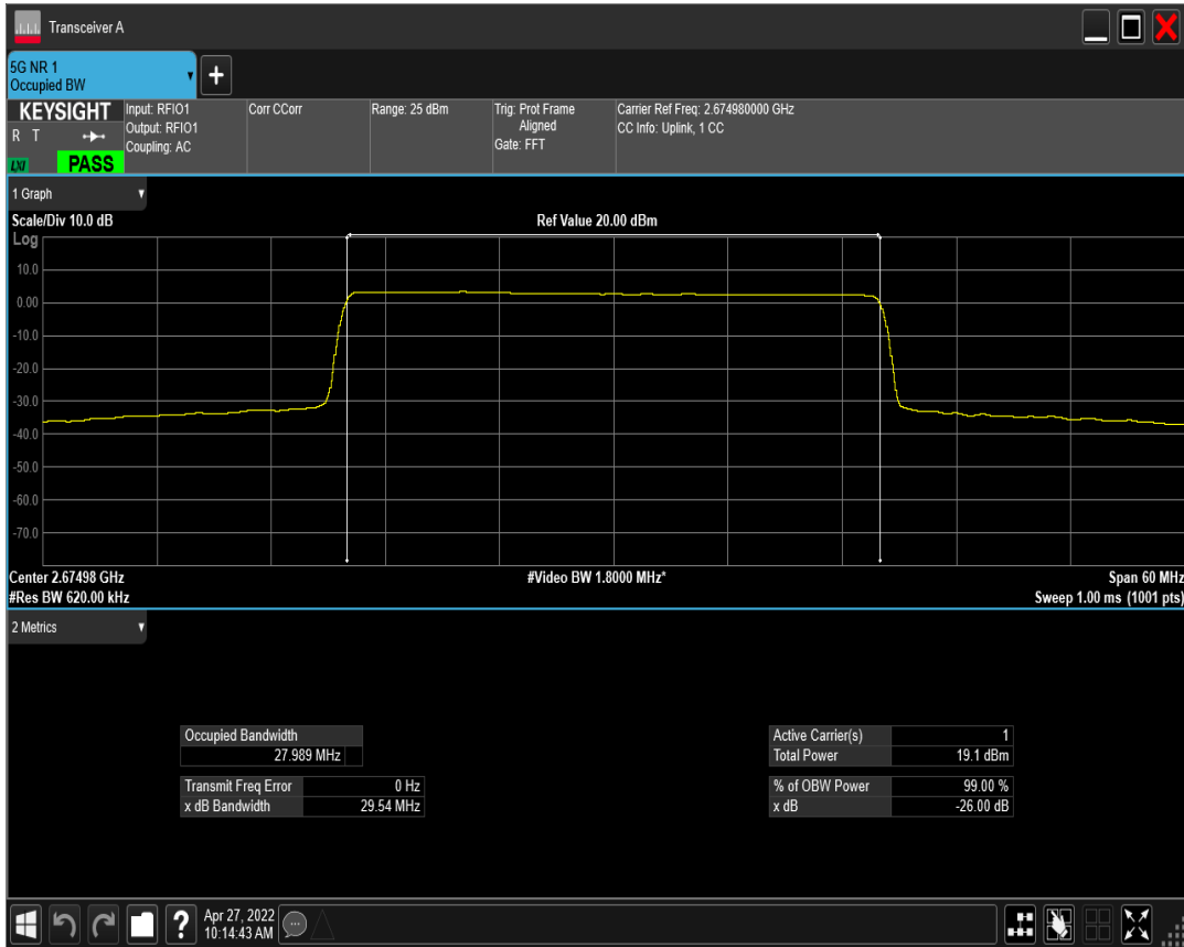
n41 SCS=30kHz CP_QPSK BW=30MHz Channel=534996 RB=78@0 ant2
