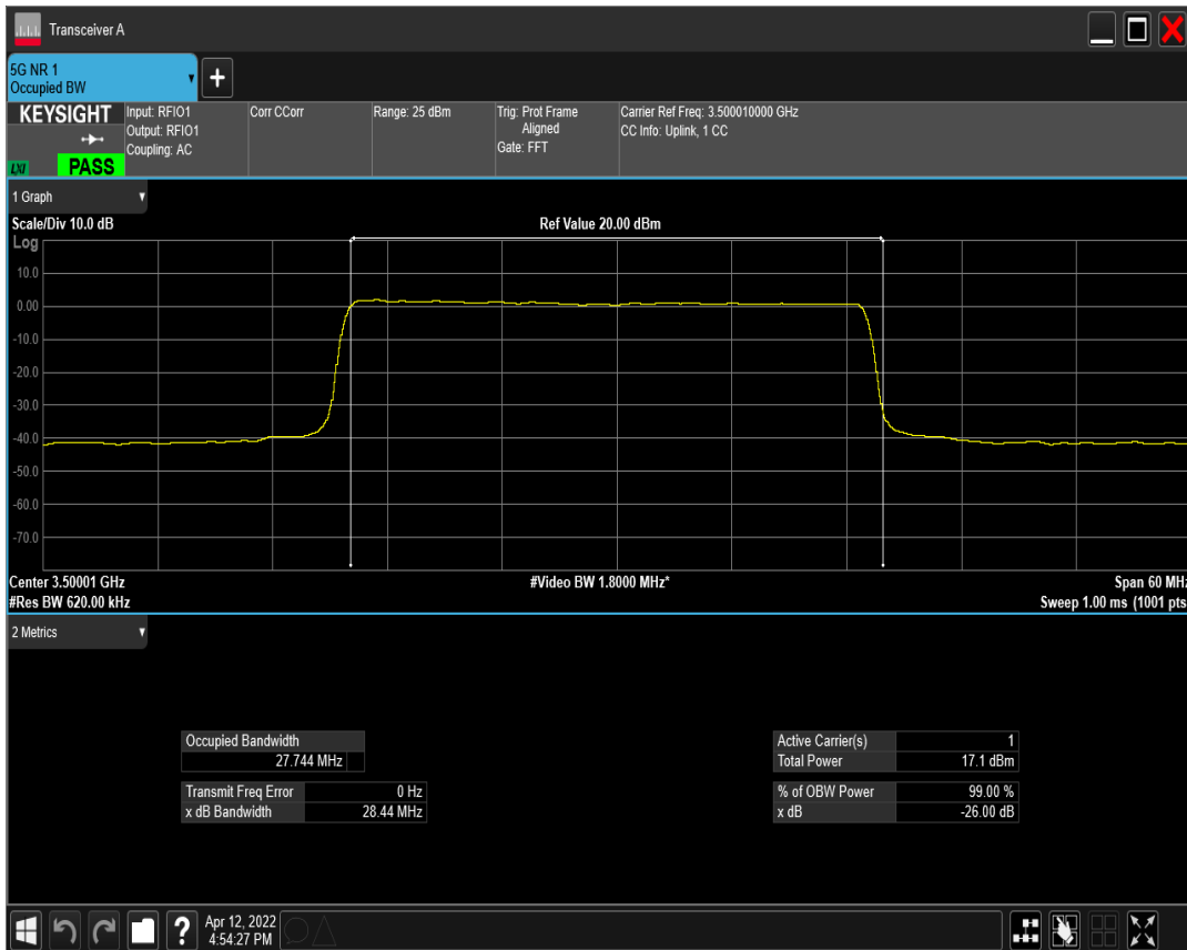
n77(3450-3550) SCS=30kHz DFT_QAM16 BW=30MHz Channel=633334 RB=75@0
