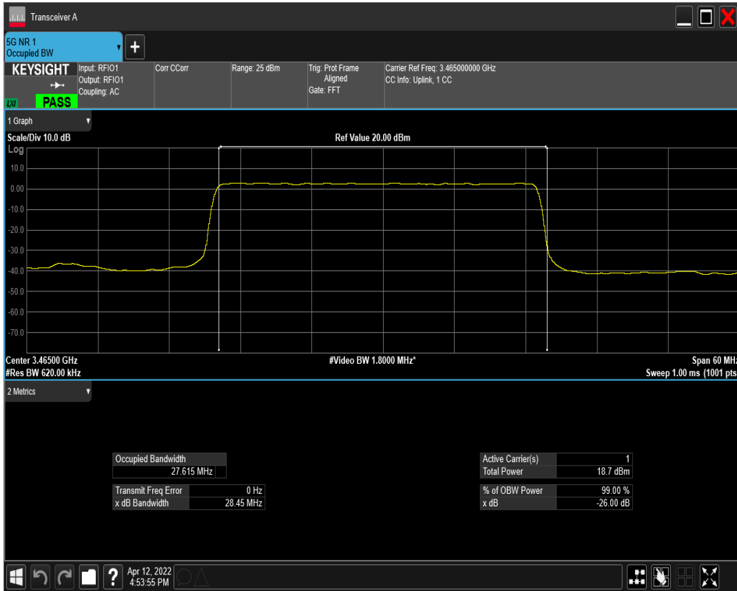
n77(3450-3550) SCS=30kHz DFT_QPSK BW=30MHz Channel=631000 RB=75@0
