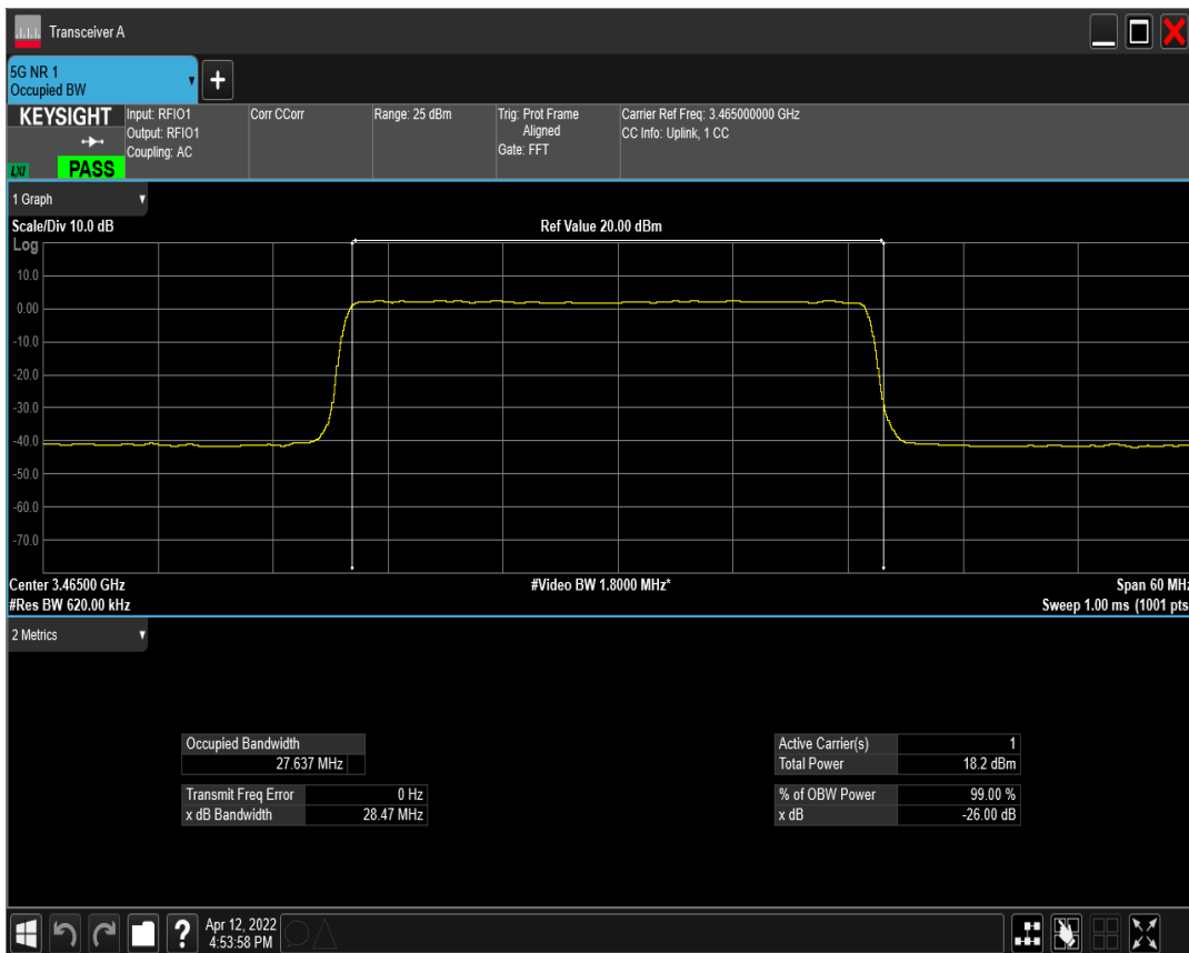
n77(3450-3550) SCS=30kHz DFT_QAM16 BW=30MHz Channel=631000 RB=75@0
