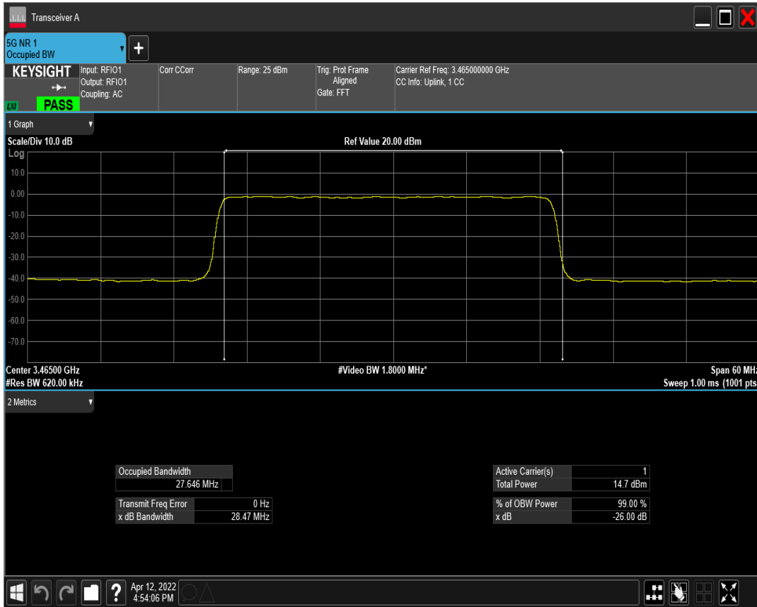
n77(3450-3550) SCS=30kHz CP_QPSK BW=30MHz Channel=631000 RB=78@0
