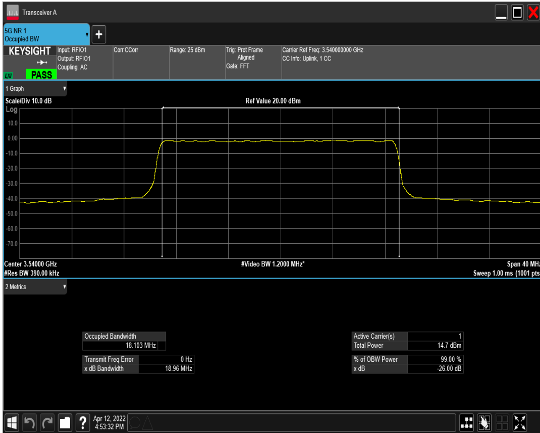
n77(3450-3550) SCS=30kHz DFT_QAM64 BW=20MHz Channel=636000 RB=50@0
