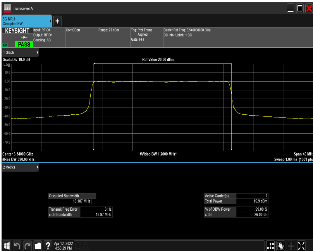
n77(3450-3550) SCS=30kHz DFT_QAM16 BW=20MHz Channel=636000 RB=50@0
