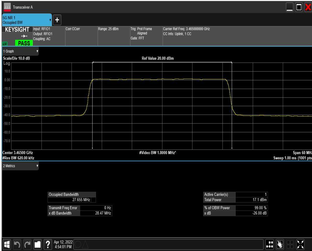
n77(3450-3550) SCS=30kHz DFT_QAM64 BW=30MHz Channel=631000 RB=75@0
