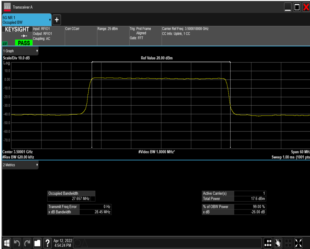
n77(3450-3550) SCS=30kHz DFT_QPSK BW=30MHz Channel=633334 RB=75@0
