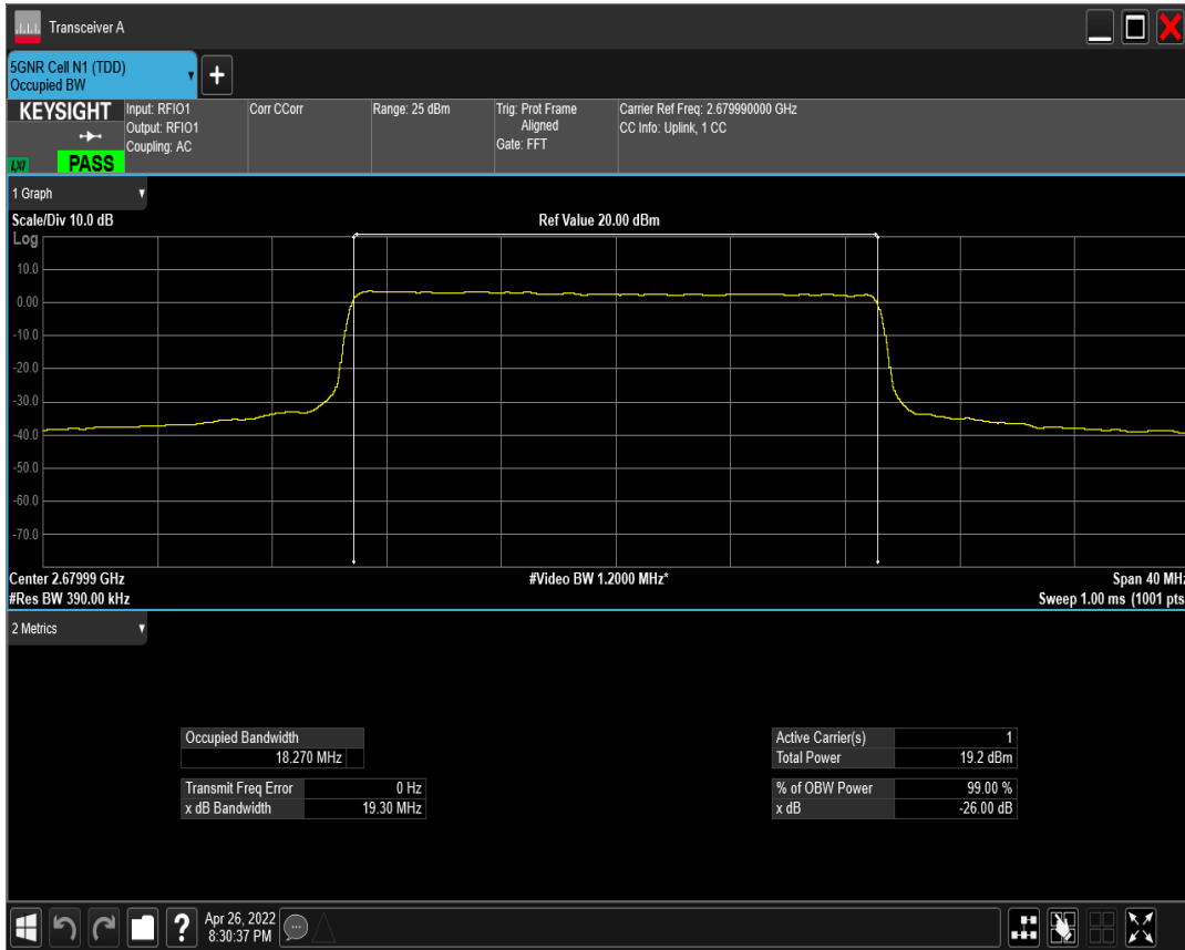
n41 SCS=30kHz CP_QAM16 BW=20MHz Channel=535998 RB=51 @0 ant2
