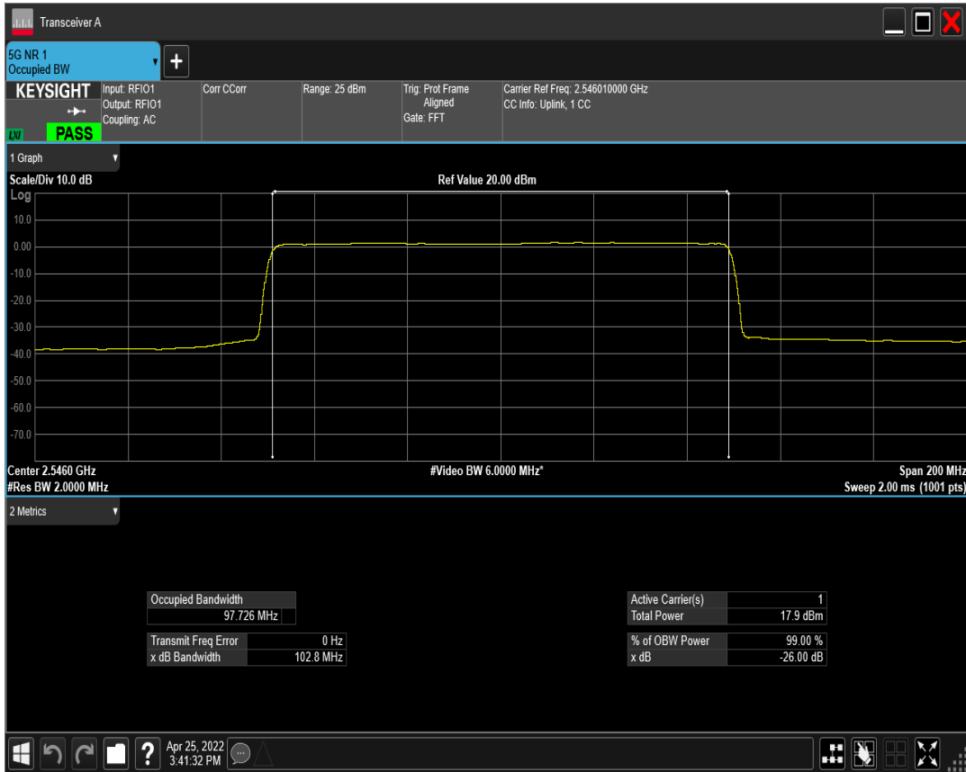
n41 SCS=30kHz CP_QAM64 BW=100MHz Channel=509202 RB=273@0 ant2
