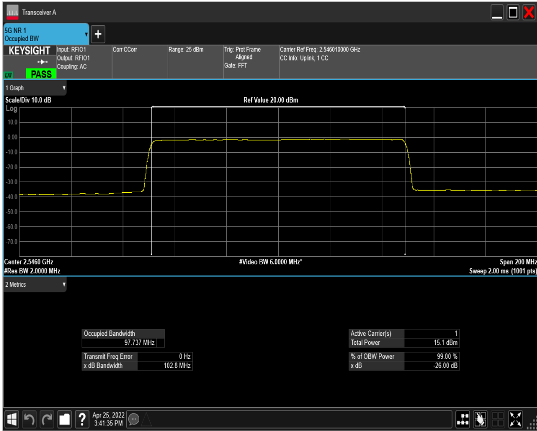
n41 SCS=30kHz CP_QAM256 BW=100MHz Channel=509202 RB=273@0 ant2
