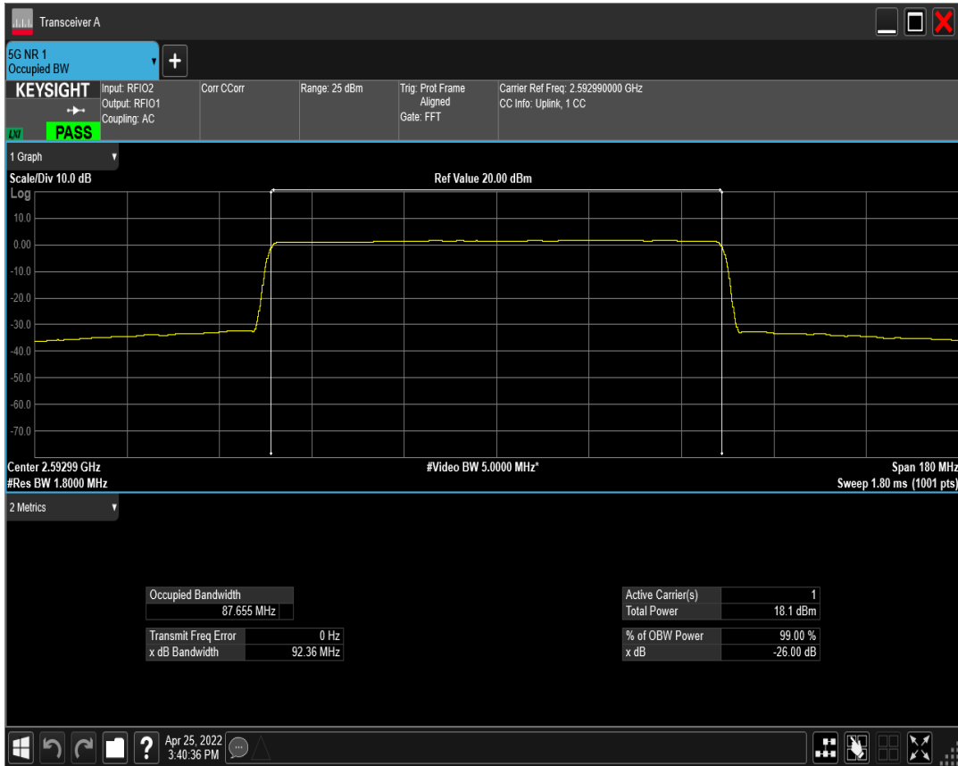
n41 SCS=30kHz CP_QAM256 BW=90MHz Channel=518598 RB=245@0 ant1
