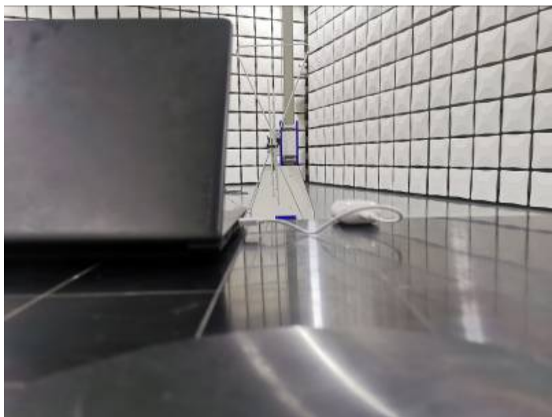
Radiated Emissions Test Setup (30-1000MHz)
