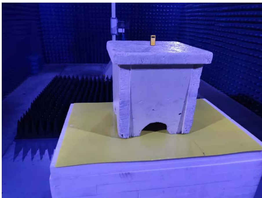
Photo of Radiated Emission Measurement Above 1GHz
