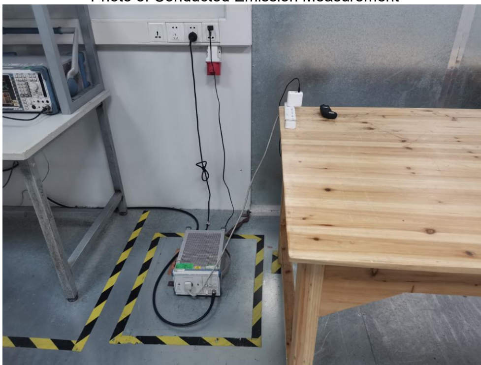
FCC ID: 2A2Z4-TERRAIN Photo of Conducted Emission Measurement
