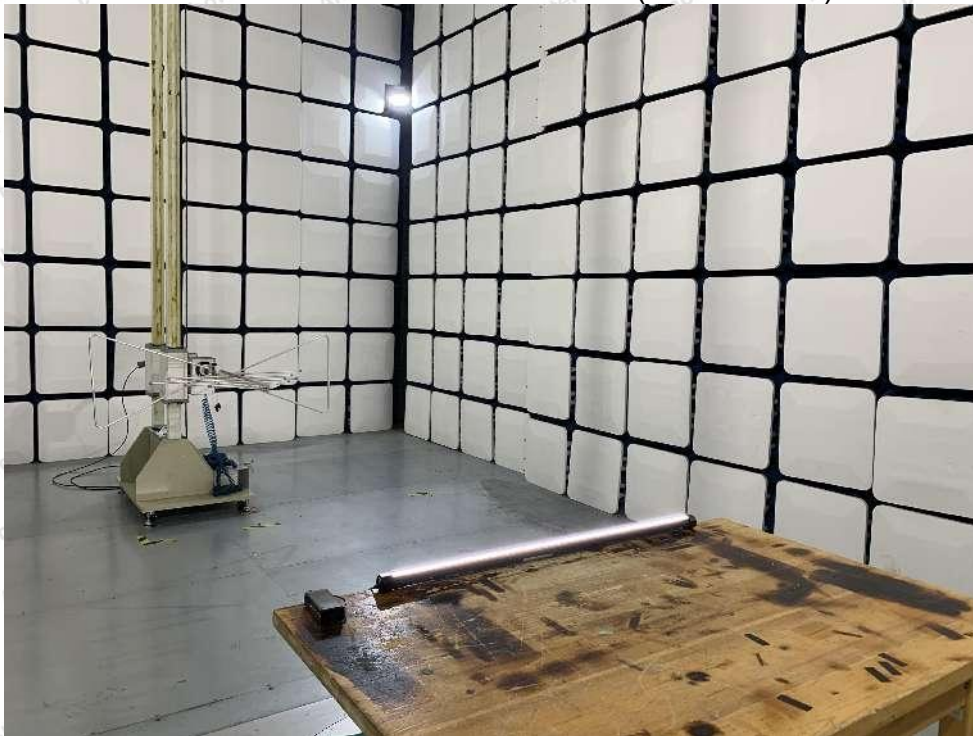
Photo of Radiation Emission Test (Below 1GHz)
