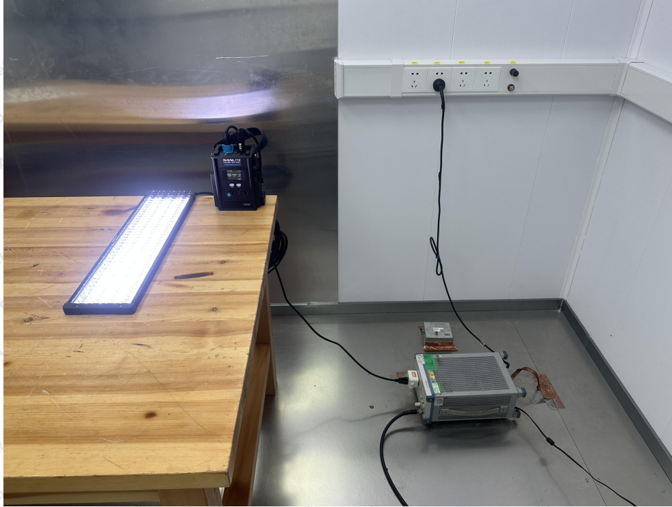
Photo of Radiation Emission Test (below 1GHz)
