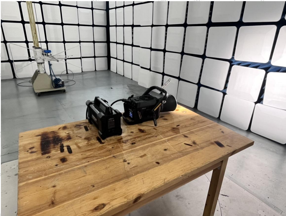
Photo of Radiation Emission Test
