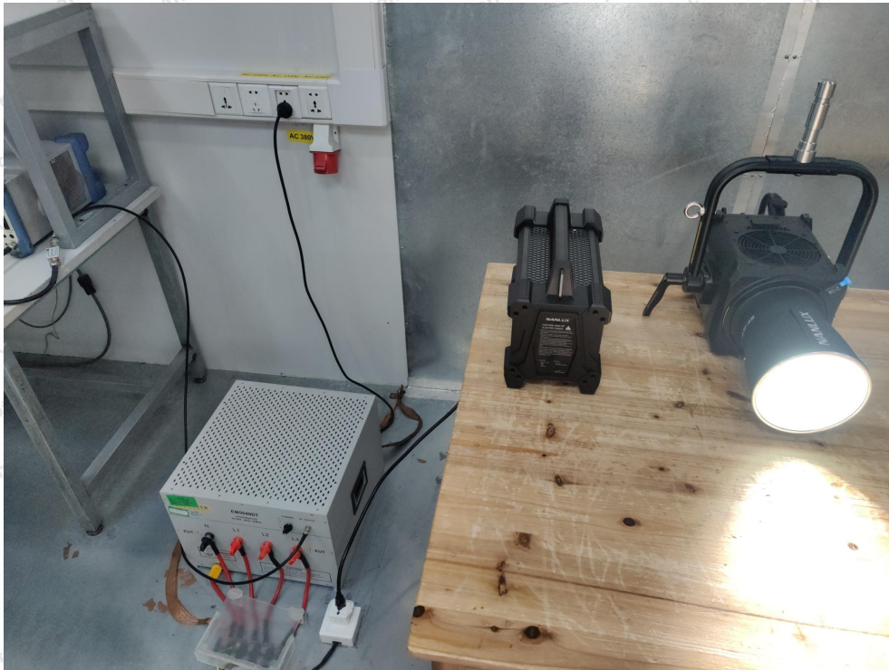
Photo of Conducted Emission Measurement
