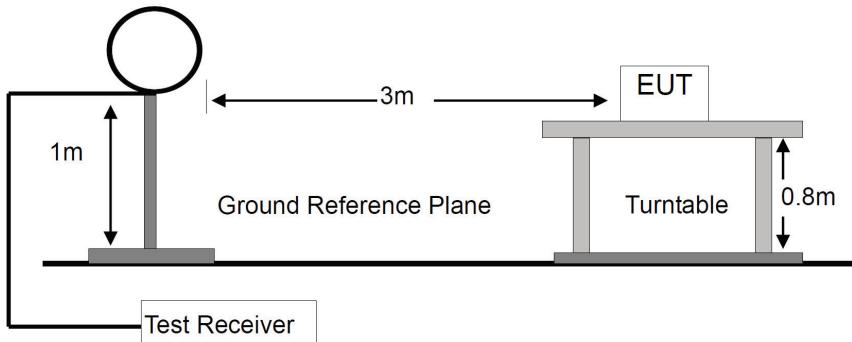
For Radiated Emission 30-1000MHz
