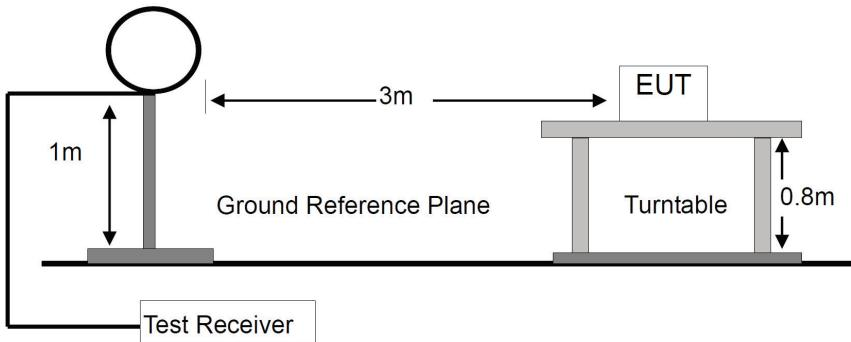
For Radiated Emission 30-1000MHz
