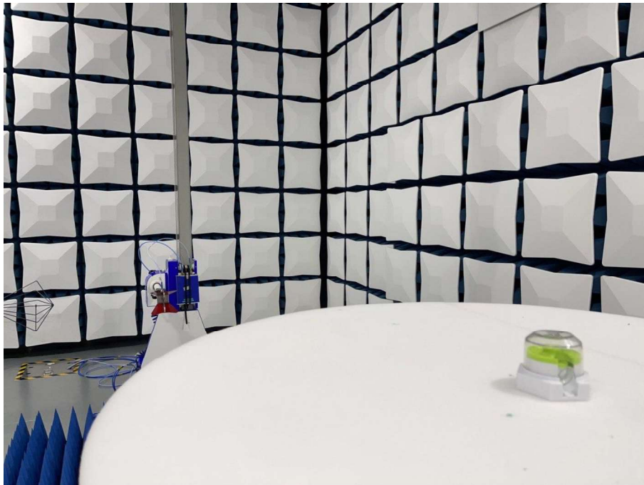
Set-up for Radiated Emission (1GHz above)
