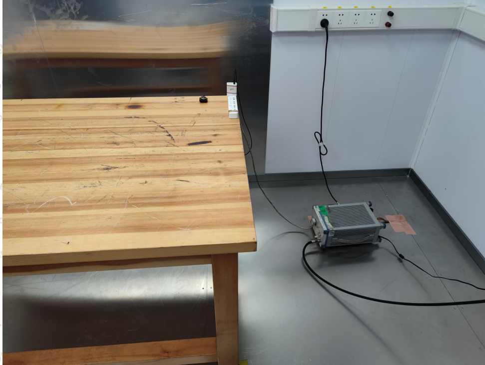
Photo of Conducted Emission Measurement
