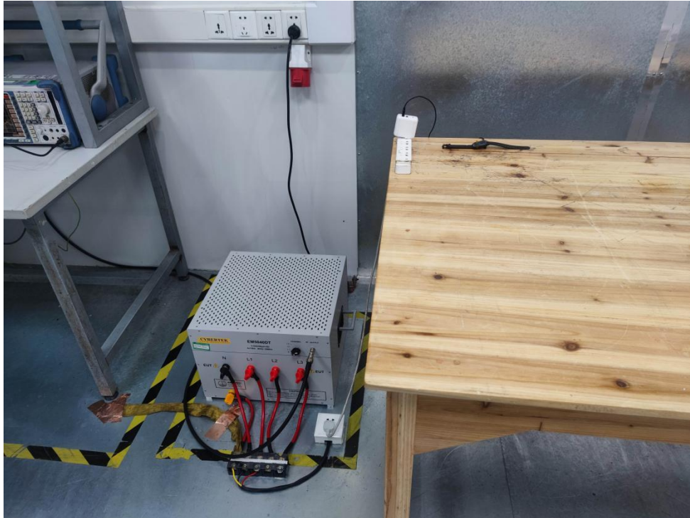
Photo of Conducted Emission Measurement
