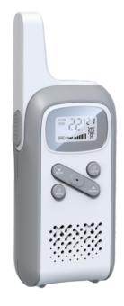
This set includes 2 walkie-talkie units: these are communication devices that operate on mobile radio frequencies. They have 8(Europe)/ 22(US) channels as well as a back-lit LCD screen, enabling you to communicate over several kilometers free-of-charge (up to 3miles in open areas).
