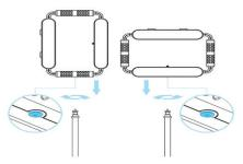
To attach a smartphone device to the Video Voyager, place your smartphone into the included phone holder, ensuring it is securely in place. Once the smartphone is secure, screw the phone holder to the inner mounting screw.
