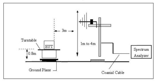
(C) Radiated Emission Test-Up Frequency Above 1GHz
