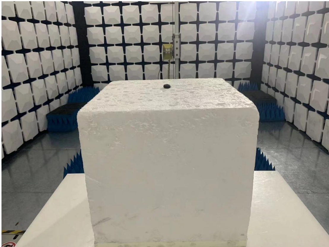
Above 1GHz for radiated emission test setup
