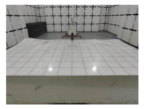
Set-up for Radiated Spurious Emission, Below 1GHz
