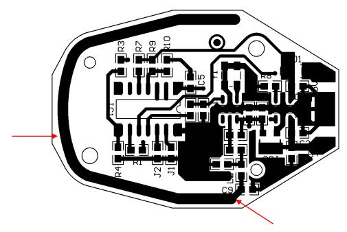
Receiver: The thick U-shaped line along the edge of the PCB pointed by the arrow is the receiving antenna, with a length of 83.6mm and a width of 1.2mm.
