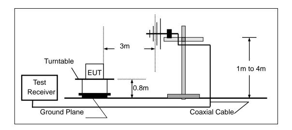
(C) For radiated emissions above 1000MHz
