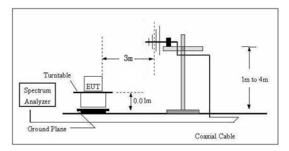
(C) For radiated emissions above 1000MHz
