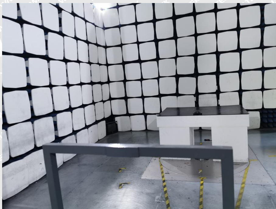
Radiation Emission Test Setup (Below 30MHz)
