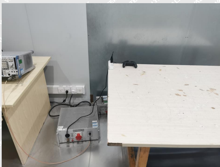
Conducted Emission Test Setup
