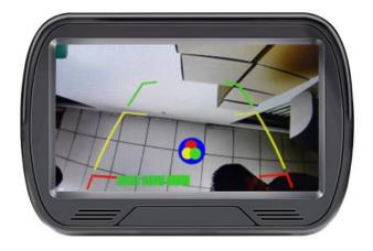
Press the Menu key three times, below picture appears, the contrast can be adjusted.
