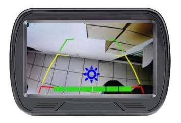
Press the menu key twice, below picture appears, and the saturation can be adjusted.
