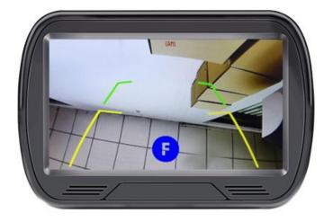
Press the menu key five times, below picture appears, the height and width of the guide line can be adjusted by press + and -
