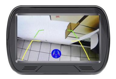
Press the menu key six times, below picture appears, and the guide lines can be moved left and right.
