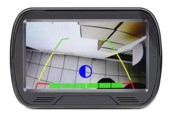
Press the menu key four times, below picture appears. The image can be flipped, normal image / mirror image. (Four forms ) by press + and -
