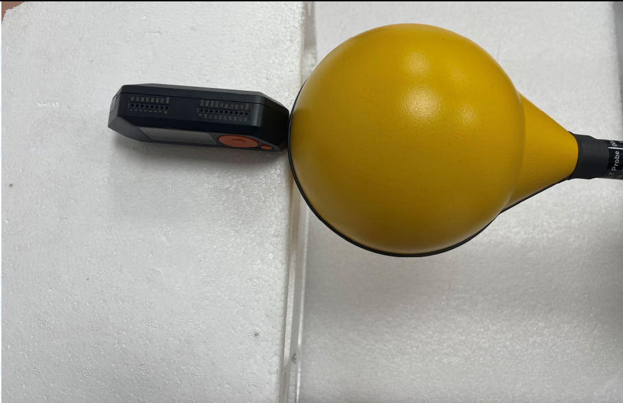
Test Position D - Exposure photo from side edge surface-Right 0mm
