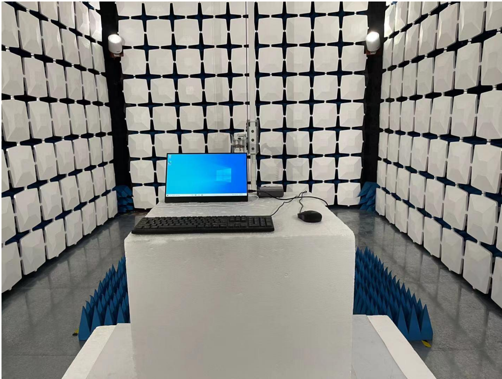
Above 1GHz for radiated emission test setup
