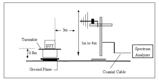
(C) Radiated Emission Test-Up Frequency Above 1GHz
