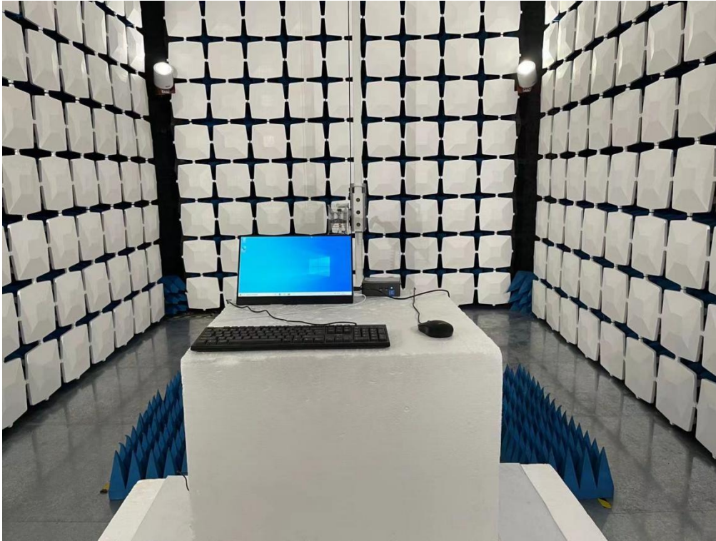
Above 1GHz for radiated emission test setup
