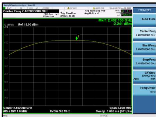
GFSK (BLE 1Mbps) LOW CHANNEL
