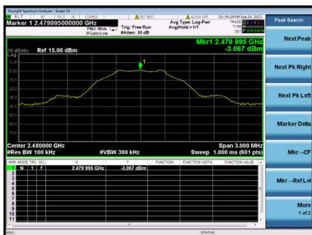
GFSK (BLE 1Mbps) HIGH CHANNEL, CARRIER LEVEL
