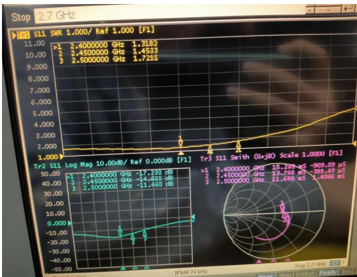
Antenna performance test diagram: (vertical polarization)
