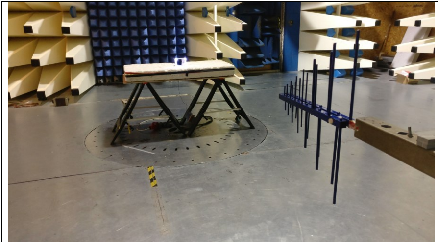
Fig 2b Test setup 300MHz -1GHz Rad Emissions
