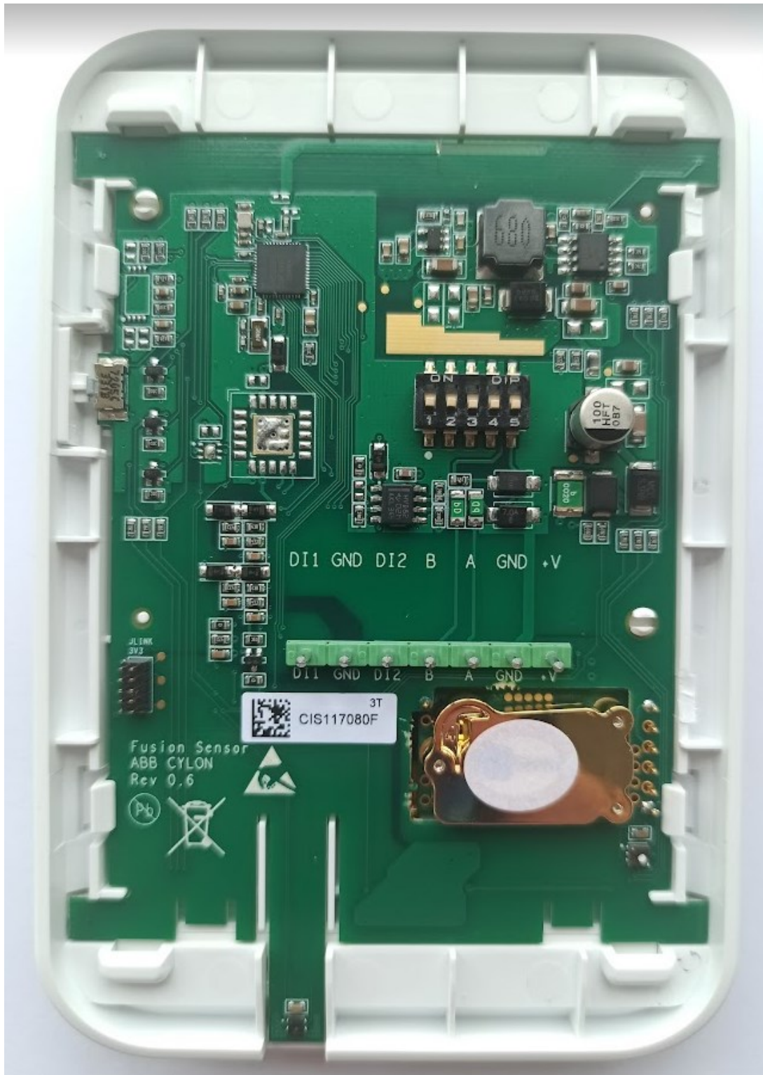
PCBA inserted in plastics
