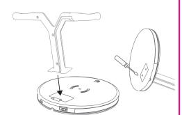
2.Insert the magnetic force of the watch into t he silicone groove
