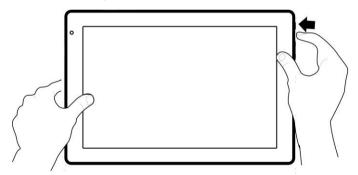
Press the power button once to access standby mode and press again to wake it up;
