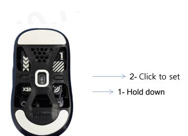
Gather Step 1: Hold the "Hz" switch and click the DPI button to switch Debounce Time. At this time, OLED will only display the current set value, other set values will be hidden; Gather Step 2: After the setting is complete, wait 1 second, OLED will return to the main i nterface:
