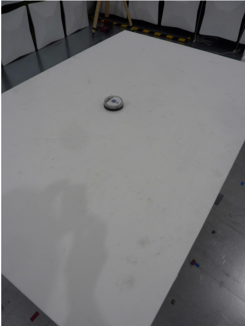
Test setup semi anechoic chamber (position 2)
