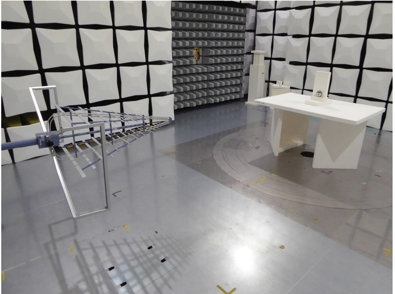
Test setup semi anechoic chamber 30 MHz – 1 GHz (Pos 2)
