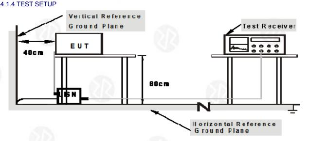
Note: 1.Support units were connected to second LISN. 2.Both of LISNs (AMN) are 80 cm from EUT and at least 8 from other units and other metal planes
