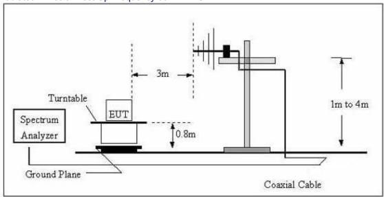
(C) Radiated Emission Test-Up Frequency Above 1GHz
