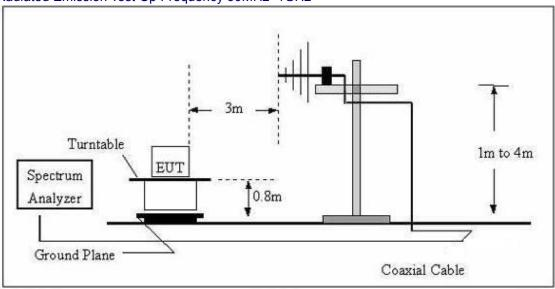
(C) Radiated Emission Test-Up Frequency Above 1GHz
