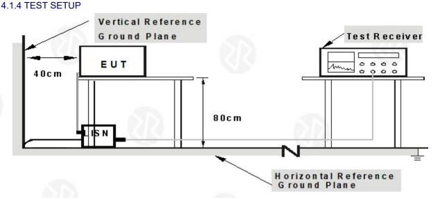
Note: 1.Support units were connected to second LISN. 2.Both of LISNs (AMN) are 80 cm from EUT and at least 80 from other units and other metal planes
