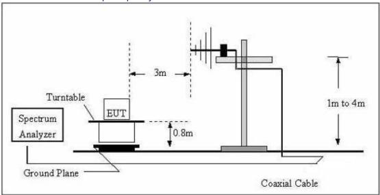
(C) Radiated Emission Test-Up Frequency Above 1GHz
