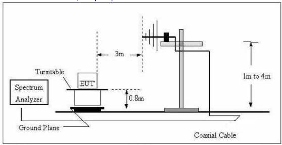
(C) Radiated Emission Test-Up Frequency Above 1GHz
