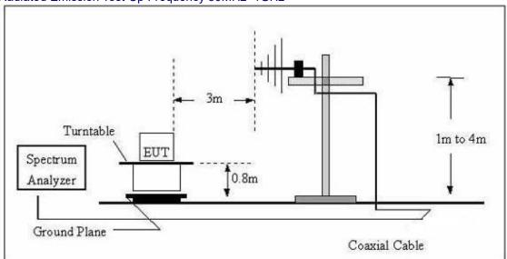
(C) Radiated Emission Test-Up Frequency Above 1GHz
