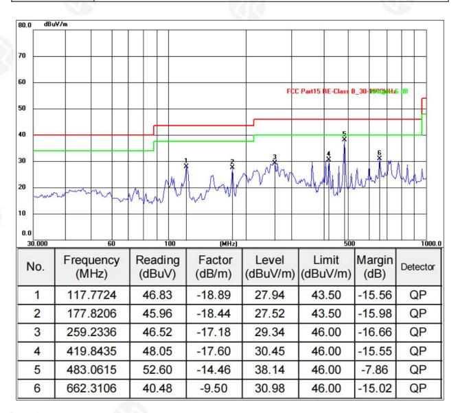
1. Final Level = Receiver Read level + Antenna Factor + Cable Loss - Preamplifier Factor
