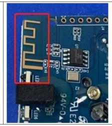
The antenna is PCB antenna. The best case gain of the antenna is 1.5 dBi.
