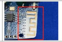
The antenna is PCB antenna. The best case gain of the antenna is 1.5 dBi.
